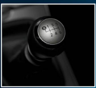
1ST GEAR - 0 TO 10MPH 2ND GEAR - 10 TO 20MPH 3RD GEAR - 20 TO 30MPH 4TH GEAR - 30 TO 40MPH 5TH GEAR - 40 TO 60MPH 6TH GEAR - 60+ MPH
